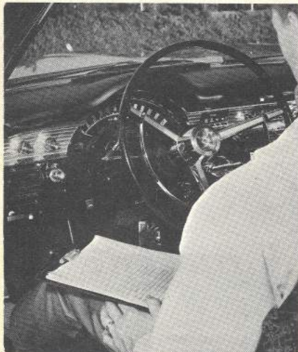
Instruments are easily visible, controls close at hand. Vent at end of dash is air conditioner.
