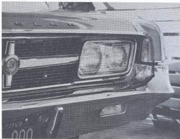
The 300-L's front silhouette is low and flat, an effect that is enhanced by repeating the grille shape in the unusual safety glass covers over the quad headlights.
